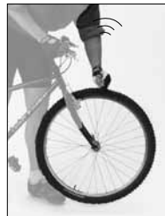
FIGURE 42: Test for loose condition
