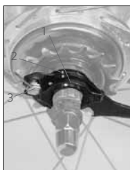
FIGURE 24: Nexus rear hub 1. Pulley 2. Cog joint bracket 3. Cable-clamp bolt
