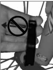
FIGURE 50: Make sure the lever does not turn
