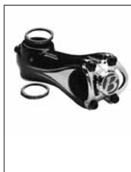
FIGURE 15: Required spacers above and below a direct-connect stem
