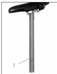
FIGURE 19: Minimum-insertion mark on seatpost 1. The bicycle frame should hide this line
