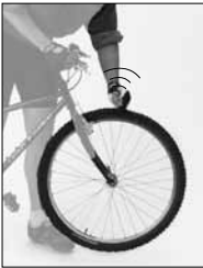
FIGURE 49: Test for loose condition
