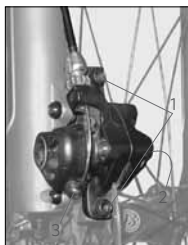
FIGURE 31: Disc brake parts 1. Attachment bolts 2. Fixed-pad adjuster 3. Cable-clamp bolt
