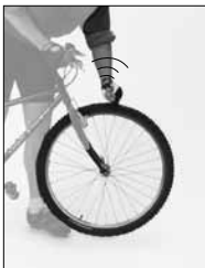
FIGURE 4: Test for loose condition
